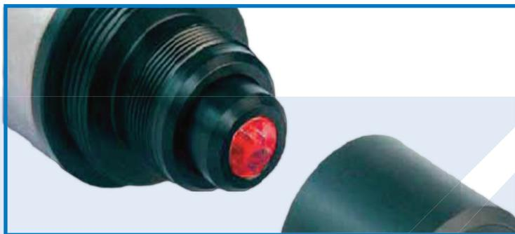
Oxygen level, water temperature, and air pressure are used by the sensor to calculate various dissolved oxygen values. The signal, then transmitted to the LXT330 universal transmitter via digital communication, unaffected by RFI and EMI noise. The optical dissolved oxygen sensor is unaffected by flow, pH, salinity, dissolved solids of the sample. While flow is not necessary, optical DO sensor can also accommodate high flow samples.
