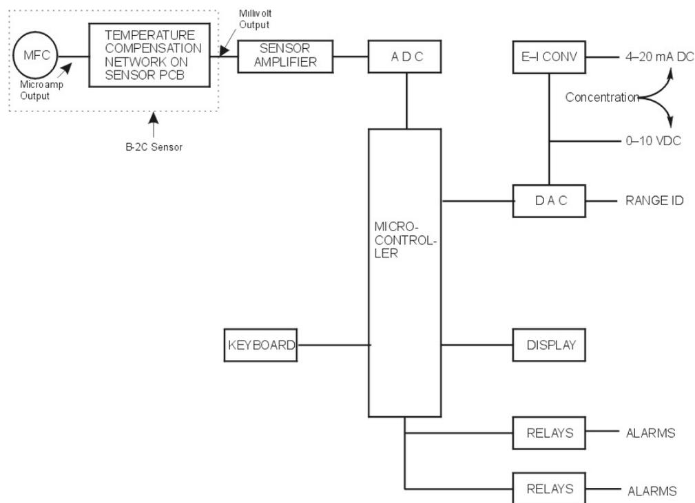
Figure 2-3: Block Diagram of the Signal Processing Electronics
