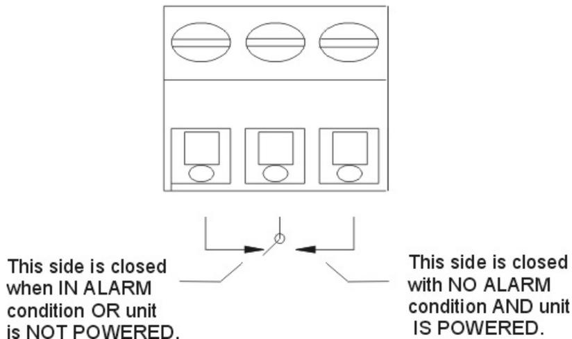
Figure 3-2: Contact ID for FAILSAFE Relay Operation
