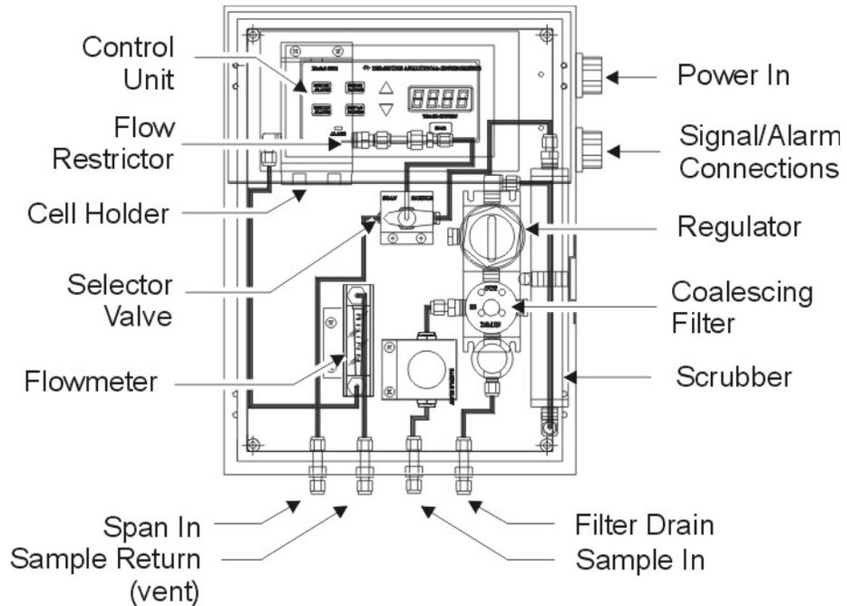
*Figure 3-3: Gas Connections*
