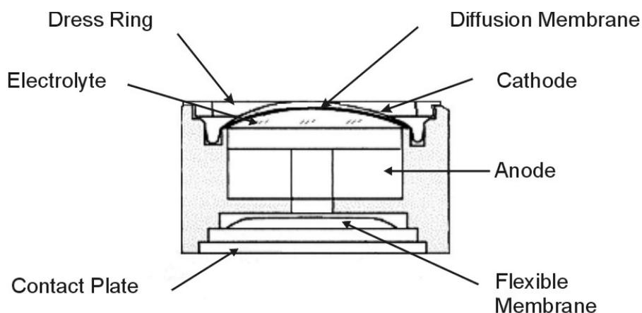
Figure 2-1: *Cross Section of a Micro-fuel Cell*
