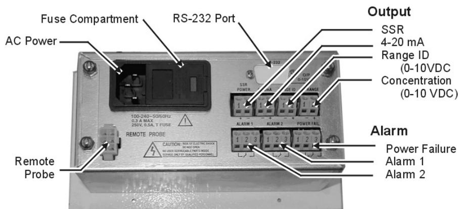
Figure 3-1: Electrical Connectors for AC Control Unit
