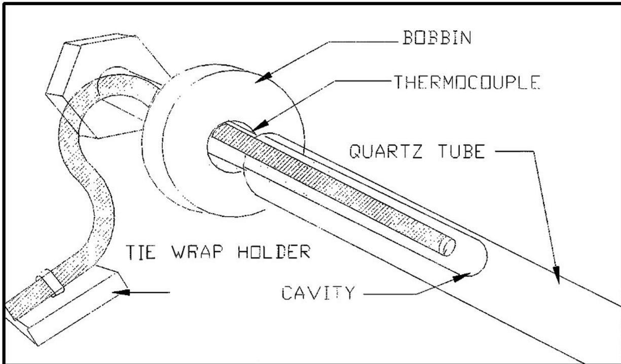
13. Reconnect the Teflon fitting that was removed earlier from the end of the quartz tube. Take care not to put any stress on the quartz tube as the Teflon fitting is tightened
