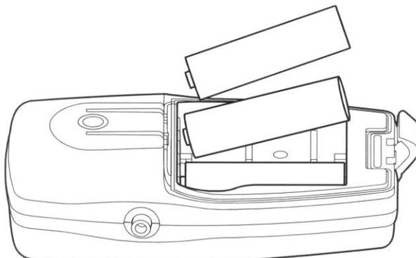
Figure 2-6: Installing Batteries
