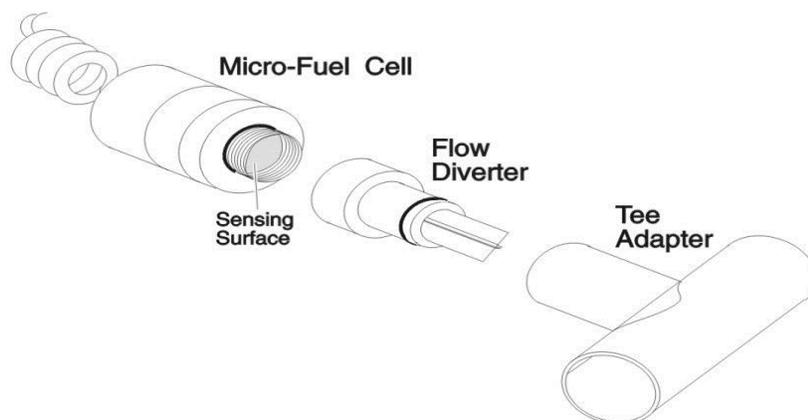
Figure 2-3: Mounting the Sensor in the Tee Adapter
