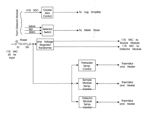
Figure 2-3. Power Module - Block Diagram
