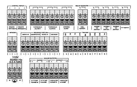
Figure 2-3: Interface Panel of the Model 6600 Control Section
