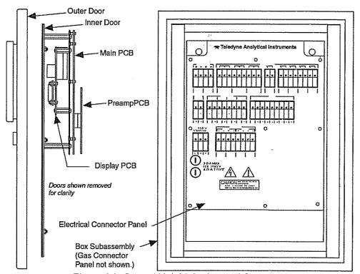
Figure 4-3: Control Unit Major Internal Components
