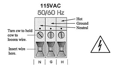
Figure 2-4: Primary Input Power Connections
