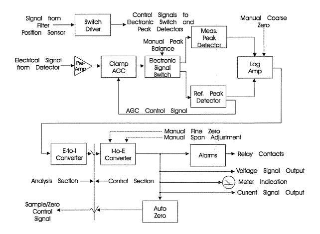
Figure 2-2 Analyzer System-Block Diagram
