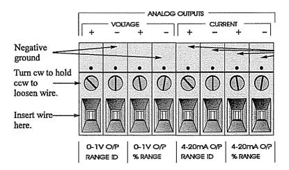
Figure 2-5: Analog Output Connections
