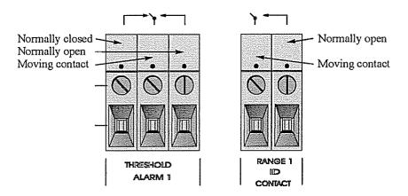
Figure 2-6: Types of Relay Contacts
