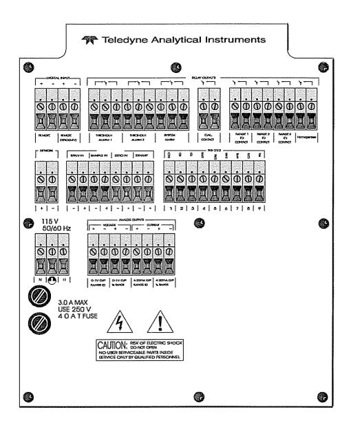
Figure 1-2: Model 6000BF Interface Panel
