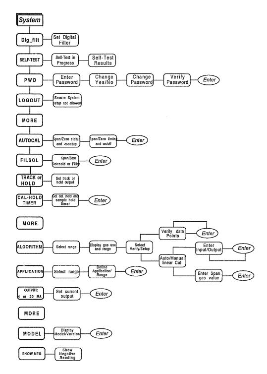
Figure 3-1: Hierarchy of System Functions and Subfunctions
