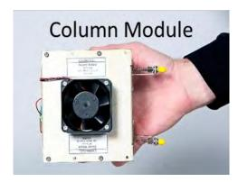
Resistively heated column modules
