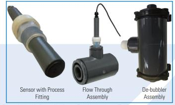
The SP3-TSS sensor is a 1" 0.D. sensor that is suitable for immersion, flow through installation. For low range Turbidity or suspended solids, flow through cell with De-bubbler assembly is required. The application with <30 NTU is calibrated inside the flow cell to ensure best accuracy. Sensor cable from 10 ft up to 30 ft. is available for various installation requirements.
