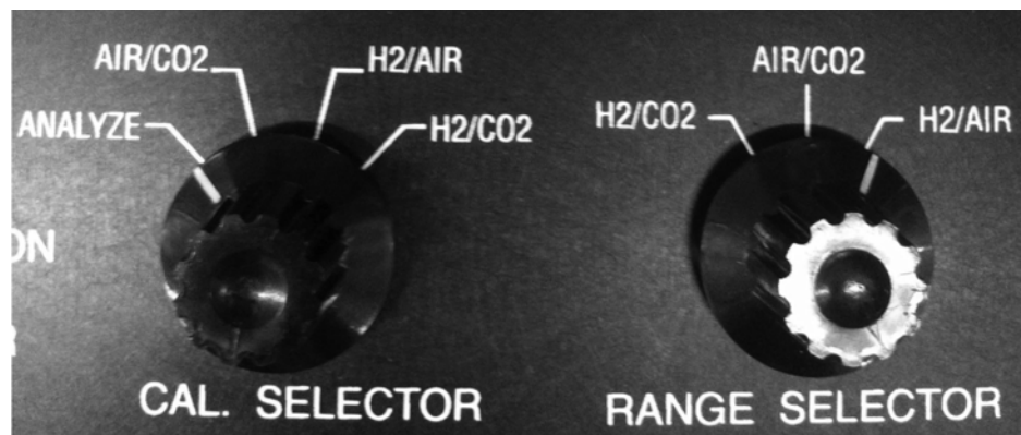
Figure 3-12: Range Switch in H 2 /AIR Position
