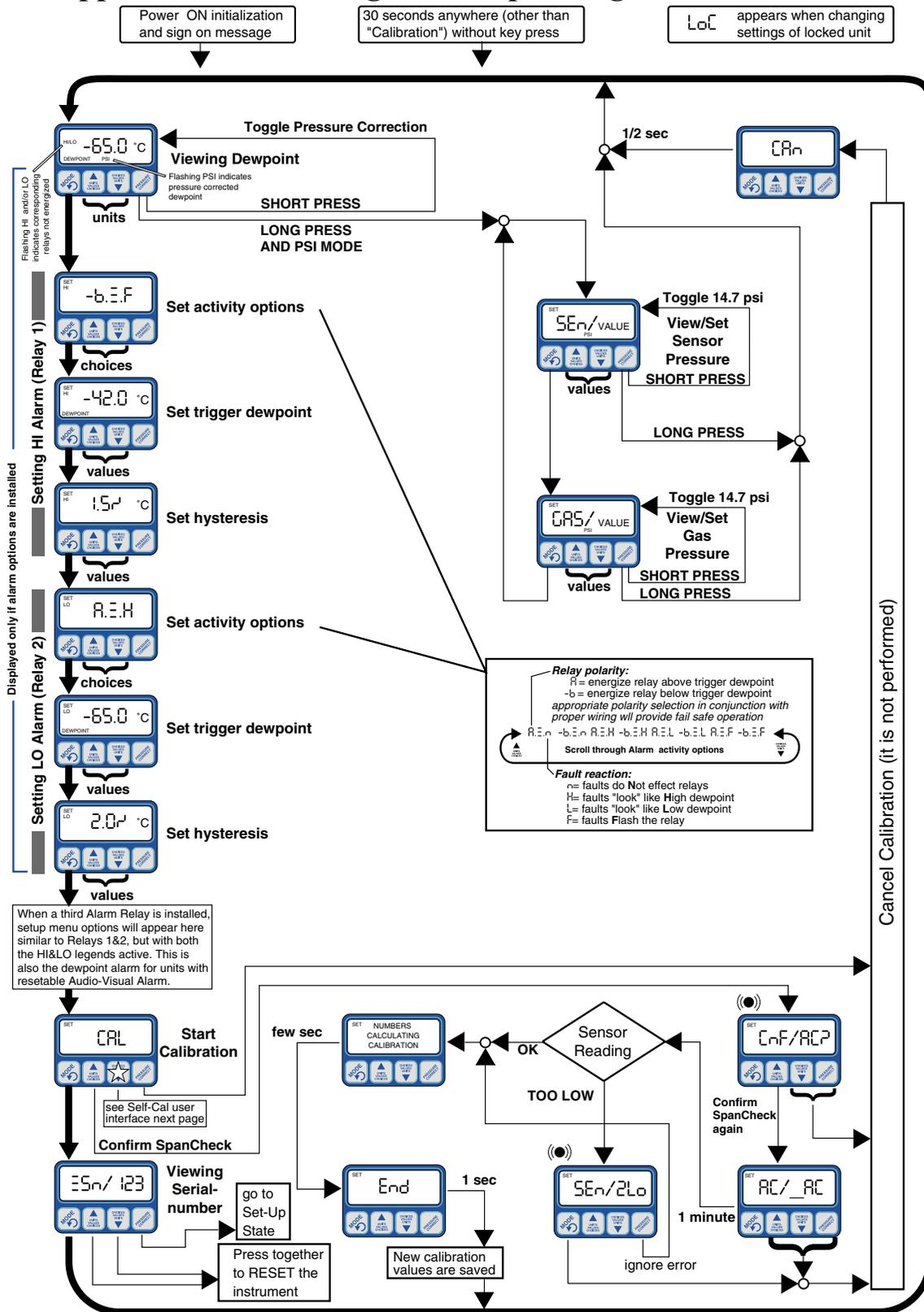
**Legend:** A slash '/' in the display area, is used to depict two alternately shown (flashing back and forth) messages. (●) denotes beeping. Buttons without designator or arrow leading out, perform no function
