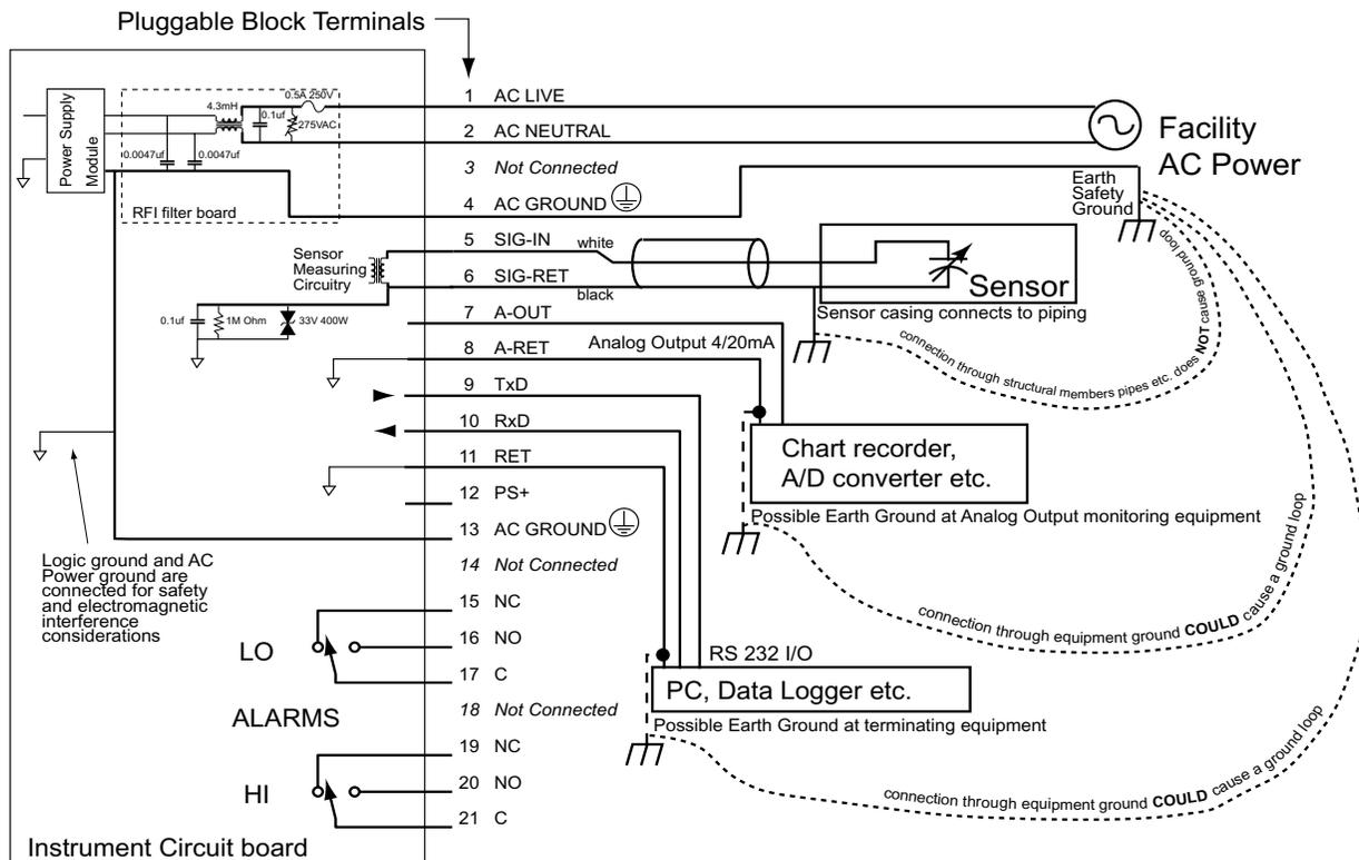
1. The sensor ground is isolated from the signal and frame grounds, however it is shunted to frame ground with a 33V Transient Voltage Suppressor, 1M Ohm resistor and 0.1uF capacitor to prevent electrostatic buildup and noise pickup. When the sensor is connected to equipment which is grounded to earth ground (because of pipes etc.), there is no ground loop because the sensor is not connected to the earth ground on the circuit board.
