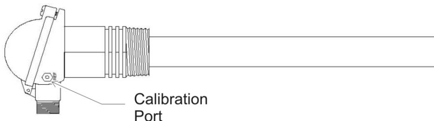
Figure 4-2: Calibration Port on Probe Head
