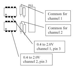
If the voltage on pin 3 goes from 0.4 to 2.0 when an auto-cal is performed the fault will be on the 9060-2 PCB.
