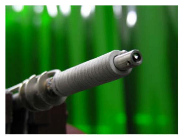
3.5.5 Gently twist the heater to and fro while sliding it off the sheath.
