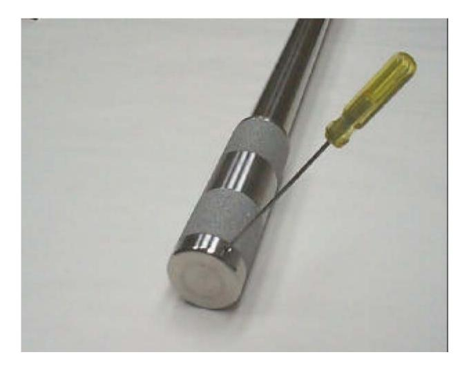
3.2.2 Slide the end cap, filters and spacer from the probe.
