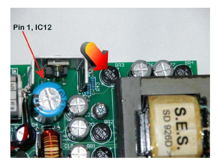
3.1.3 On analysers with version 1.6 or earlier 1630-2 boards, the 40-way ribbon cable is worn or damaged. Measure the 5V rail on the 1630-2 PSU board and then on the 1630-1 board. If the value measured on the 1630-1 board is less than the value measured on the 1630-2 then the ribbon cable is causing excessive voltage drop.
