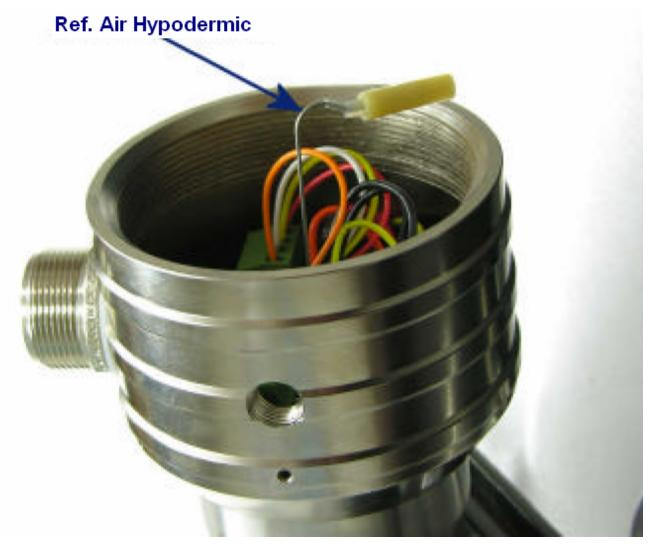
3.3.3.5 Remove the reference air hypodermic by lifting straight up. Do not bend. Sharp bends could cause a blockage in the tube.
