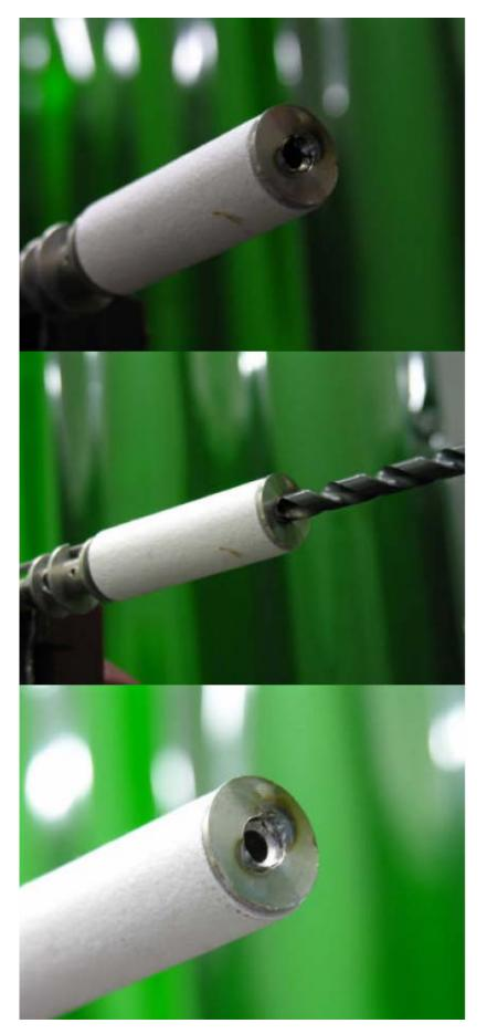
3.6.3 Use multi-grips to remove the heater insulation retainer.
