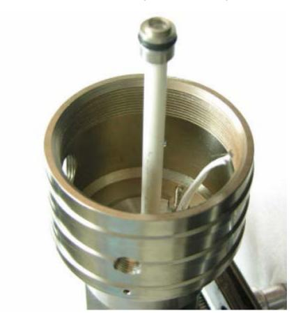
3.3.5.5 Carefully insert the four-bore assembly into the sensor.
