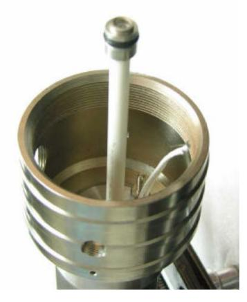
3.3.3.18 Remove the probe head from the probe body by unscrewing the two retaining screws.
