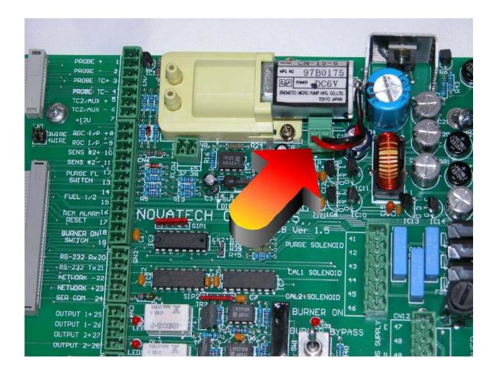
3.1.2 The bridge rectifier, BR3, has an open circuit diode reducing the available power from the 5V rail. This can be confirmed measuring the pre-regulated DC voltage on pin 1 of IC12, this should be between 14 & 18VDC, or by using a CRO. Replace BR3 and make sure the component is installed so there is at least 3mm between the component and the circuit board. This helps the component to dissipate heat.
