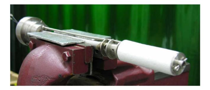
3.6.2 Use a 3/8" drill to break the weld on the heater insulation retainer.
