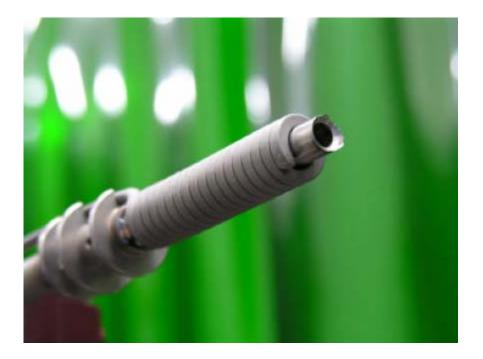
3.6.5 Gently twist the heater to and fro while sliding it off the sheath.
