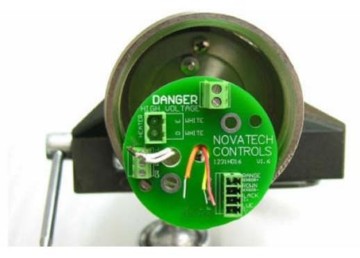
3.3.5.7 Replace both circuit board retaining nuts and flat washers.
