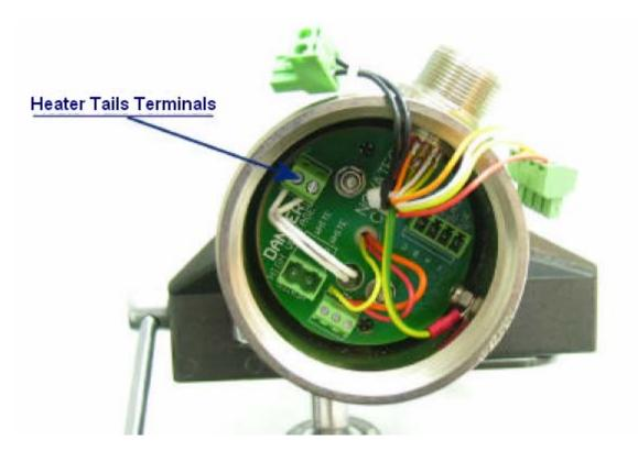
3.3.5.12 Plug in the two wire heater connector and four way sensor / T/C connector.
