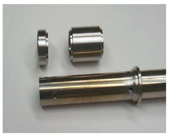
3.2.5 Reassemble the filter assembly. The grub screws on the filter retainer should engage the grub screw locking holes at the end of the outer sheath.
