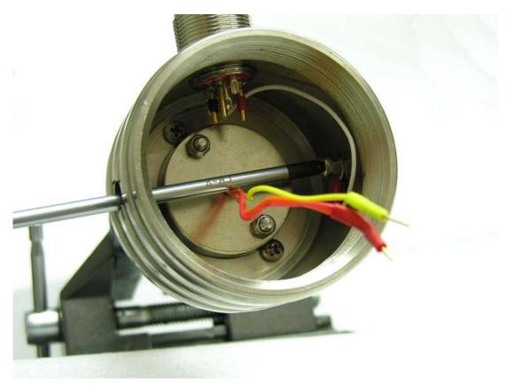
3.4.1.6 Evenly remove the two Nylok nuts holding down the compression plate. This will remove the spring loading on the four-bore insulator and the sensor.
