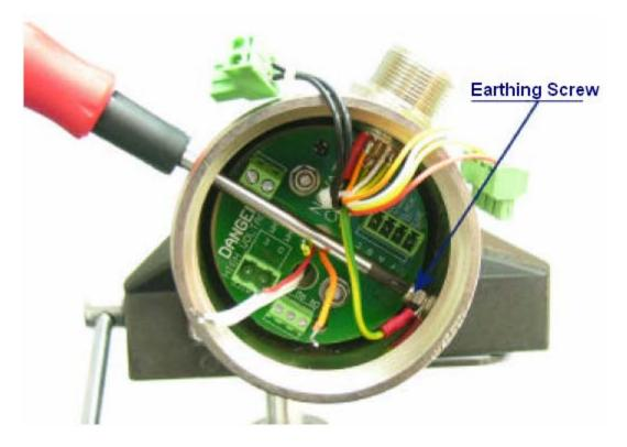
3.3.5.10 Replace the O2 +ve (orange), T/C +ve (yellow) and T/C –ve (red) into the three way terminal block. The terminals are marked "O", "R", and "Y".
