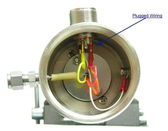
3.4.1.4 Remove the silicon tube from the hypodermic that runs through the head connector or from the barb on the external reference air connector. (Gently work the silicon tube to get this off)
