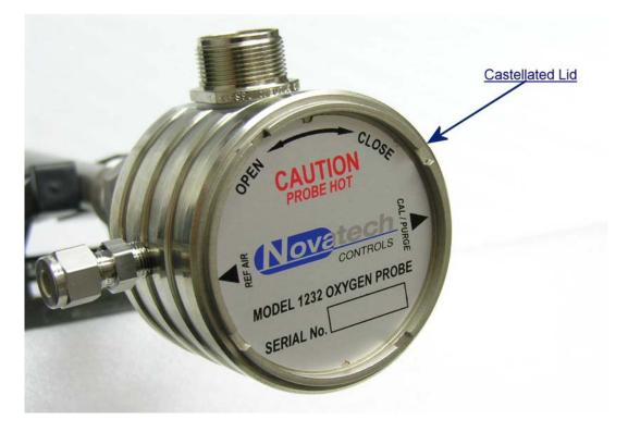
3.4.1.3 Unplug the wiring from the head connector. These are the probe positive, thermocouple positive and thermocouple negative. The thermocouple is optional in the 1232 probe.
