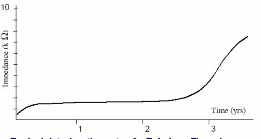
Typical deterioration rate of a Teledyne Zirconia sensor
