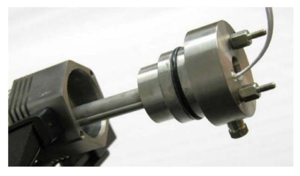
3.3.5.2 Align the reference air male connector port in the head opposite the 1/8" NPT calibration port on the inner sheath assembly; screw the probe head to the probe body with the two retaining screws.
