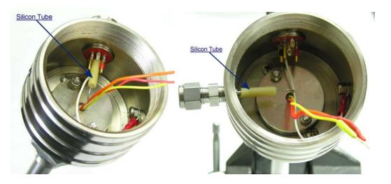
3.4.1.5 Remove the earthed wire inside the head  $(O_2 - ve)$  and remove the head connector.
