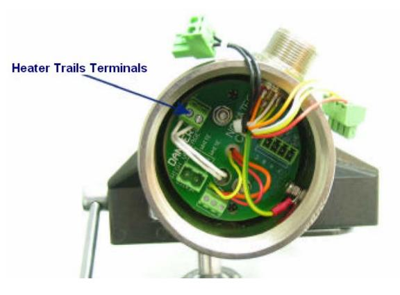
3.3.3.8 Remove the O2 +ve, T/C+ve and T/C-ve wires from the three way terminal by loosening the three screws.
