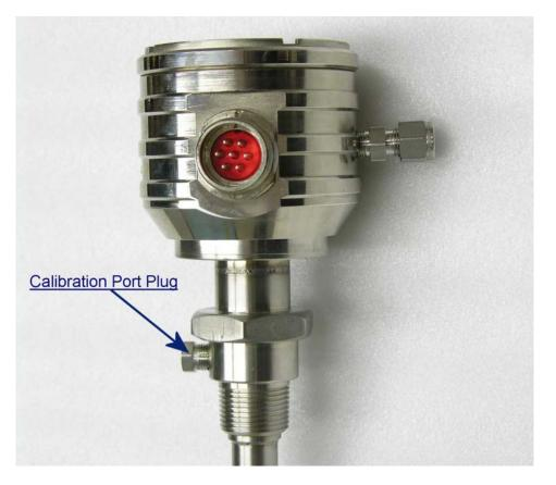
3.4.1.2 Remove the castellated lid on the probe head. Use the shank of a suitable spanner or a square cross-section bar
