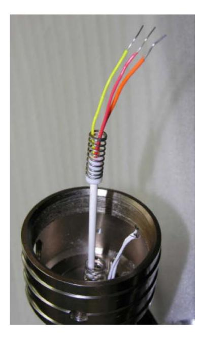
3.3.5.6 Feed the four-bore wires through the circuit board centre hole and the heater wires through the hole adjacent to the three-way connector. Install the reference air hypodermic into the four-bore insulator. While pushing the circuit board into position take extreme care lining up the four-bore spring and sensor compression spring to avoid breaking the four-bore insulator.
