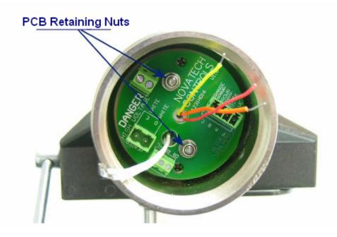
3.33.12 Lift the circuit board over the heater, O2 +ve, T/C +ve and T/C -ve wires.
