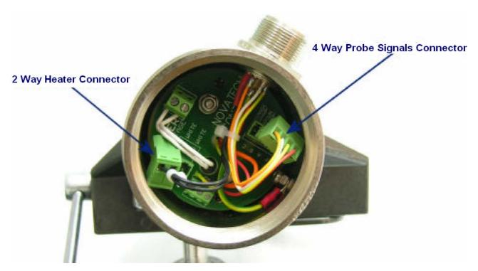
3.3.3.7 Remove the heater tail wires from the two way terminal by loosening the two screws.
