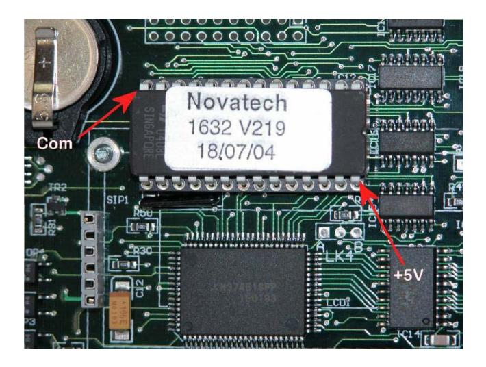
There are spare conductors in the ribbon cable that can be utilized for the 5V rail and the common of the power supply. Solder two jumpers to each of the headers as shown below.
