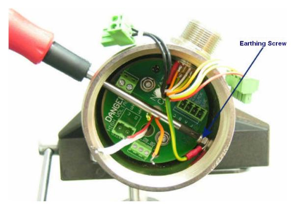
3.3.3.10 If installed, remove the weatherproof plug (head connector) by unscrewing (anticlockwise). Avoid twisting the wires while unscrewing the connector.
