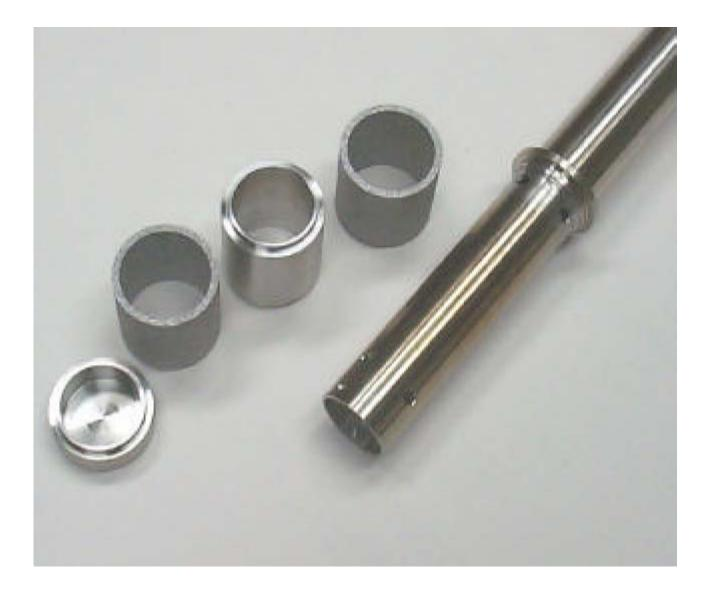
3.2.3 Use clean compressed air to dislodge any particulate that may have accumulated inside the filter assembly. If particulate build up is excessive then consider using the 15 micron filters. The finer filters will considerably dampen the response time of the probe.
