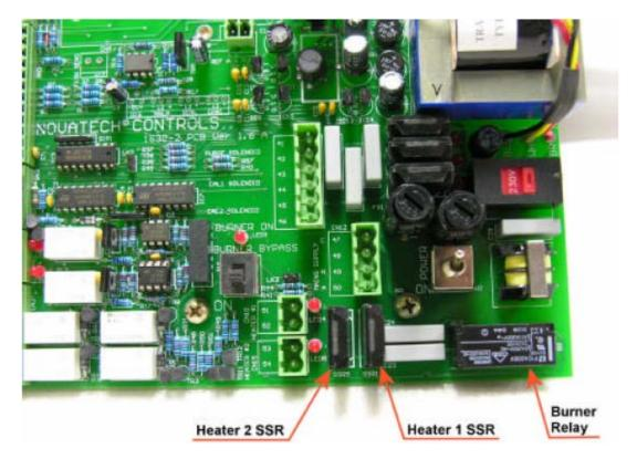
The most common mode of failure for a solid state relay is a short circuit. This will result in 100% power applied to the probe or sensor's heater that will destroy the heater due to excessive temperature.
