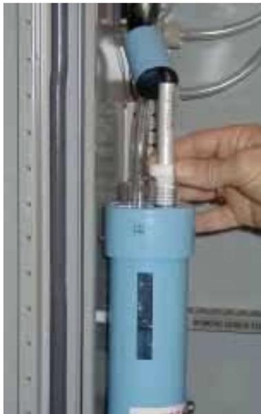
In the analyzer described there is a chemical oxidation system based on a highly concentrated sodium persulphate, catalyzed by a double wavelength UV lamp.
