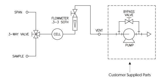
Figure 3-5: Piping Diagram for Vacuum Service Option
