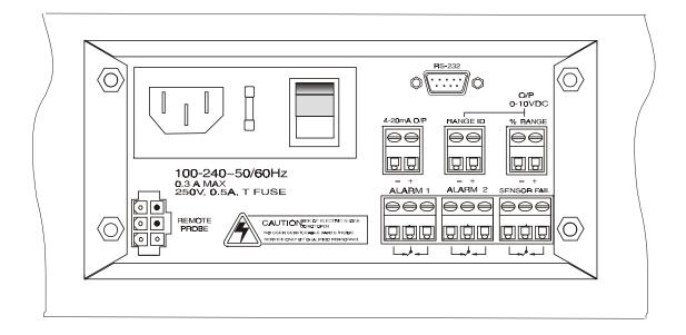
Figure 3-1 Electrical Connectors for AC Control Unit
