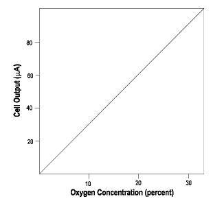
Figure 2-2. Characteristic Input/Output Curve for a Micro-Fuel Cell
