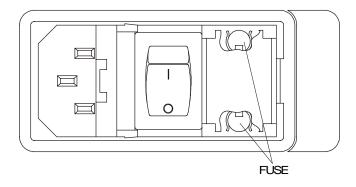
Figure 5-1: AC Fuse Replacement
