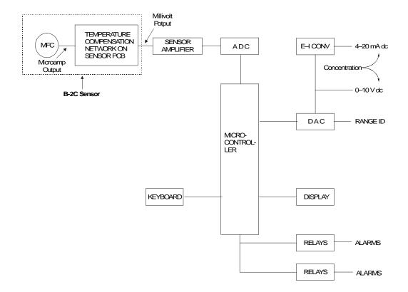
Figure 2-3: Block Diagram of the Signal Processing Electronics
