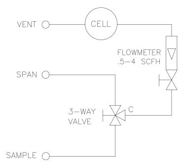
Figure 3-4: Standard Piping Diagram
