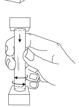
Figure 5-2: Removing/Replacing the Humidifier
