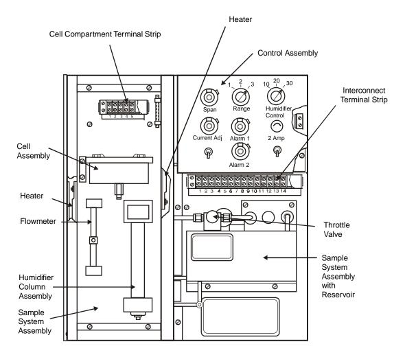
Figure 4-1: Typical Model 306WA With 2 Alarm Option
