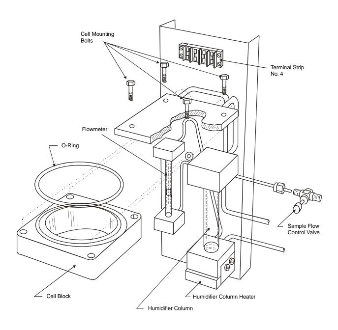
Figure 4-2: Cell Compartment Components
