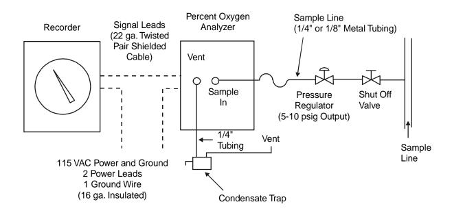
Figure 2-1 Typical System Layout
