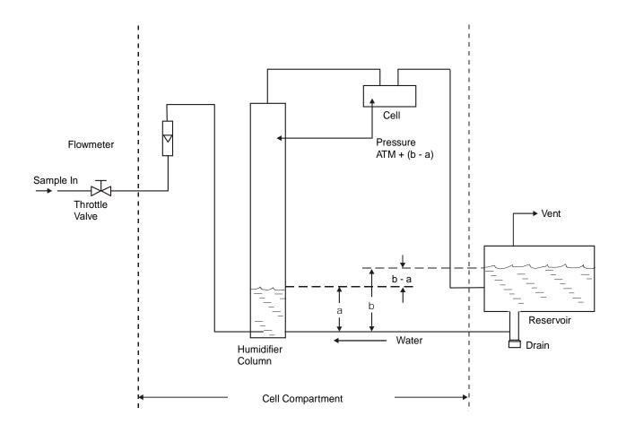
Figure 2-1: Flow System Schematic
