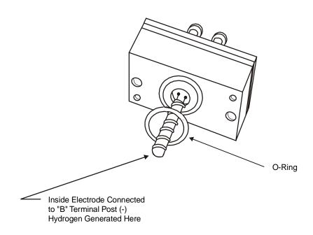
Figure 8: Calibrator Assembly
