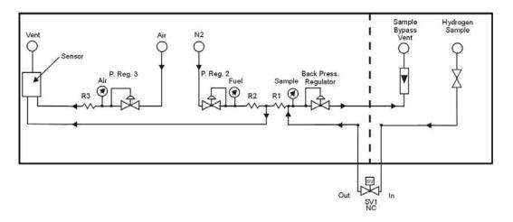
Figure 1-2: Gas Sample System Without Optional AutoCal Valves
