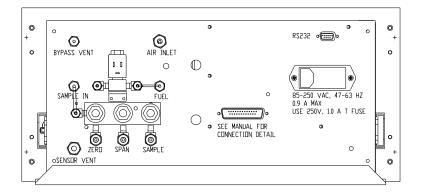
Figure 3-1: Gas Connections
