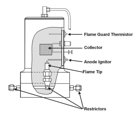
Figure 1-3: Flame Ionization Cell
