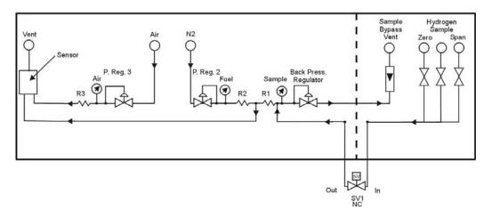
Figure 1-1: Gas Sample System with Optional AutoCal Valves
