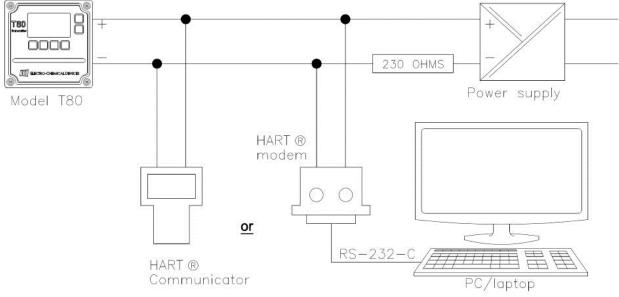
Figure 3-8: Wiring Diagram
