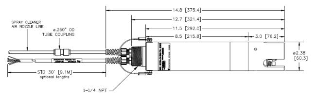
Figure F-2: Ammonium NH<sub>4</sub>-N Dimensions
