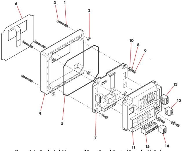
Figure 8-1: Exploded Diagram of Front Panel Control Board with Relays
