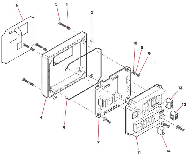
Figure 8-1: Exploded Diagram of Front Panel Control Board
