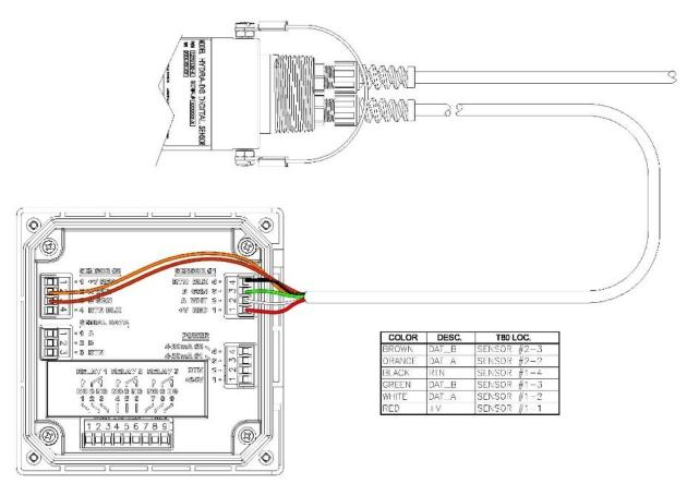
Figure F-1: Wiring Diagram Ammonium NH<sub>4</sub>-N
