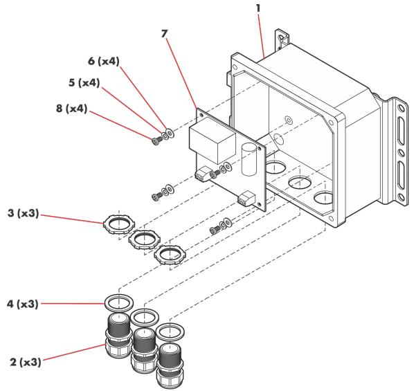
Figure 8-1: Exploded Diagram of Back of Transmitter Case with Cable Glands
