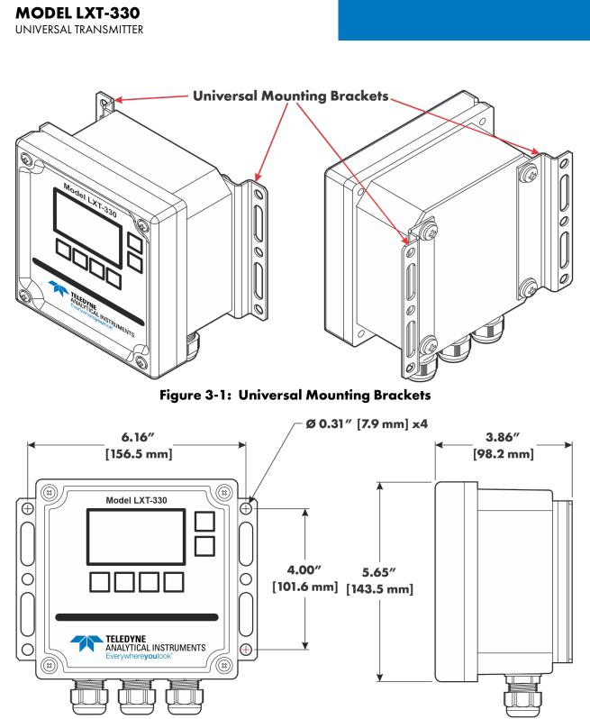
Figure 3-2: Universal Mounting Bracket Dimensions
