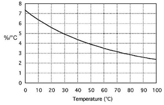
Figure D-1: % Change per °C for 18.2 MΩ Water
