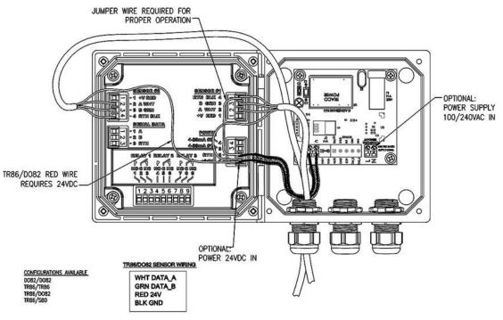
Figure 3-7: 4-Wire Transmitter
