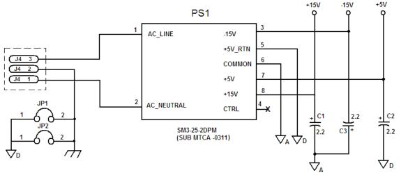
Refer the below Circuit diagram to measure the voltages on the Rear Panel Board- Power Module;
