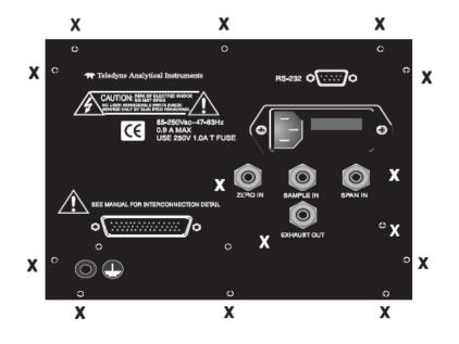
To detach the rear panel, remove only the 14 screws marked with an X. Position the rear panel assembly properly & apply the power supply to the instrument.
