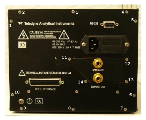
For percent oxygen analyzers such as the 3000PA and 3000MA, the fittings on the rear of the unit are connected via flexible tubing and for those units, it may be possible to leave screws 11-14 in place.
