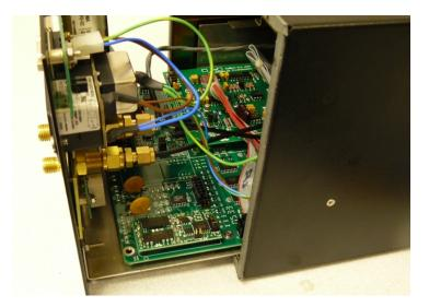
Once the screws have been removed, it will be possible to slide the rear panel away from the rest of the case. A sub assembly that consists of the rear panel and a lower metal frame to which the motherboard is attached will slide out. There are metal rails that are inside the analyzer case that guide this assembly.
