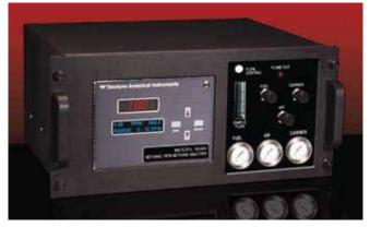
Model 4030 uses TAI's field proven FID detector in a heated chamber. The chamber is heated to a high temperature to meet US EPA requirements for VOC emissions monitoring.
