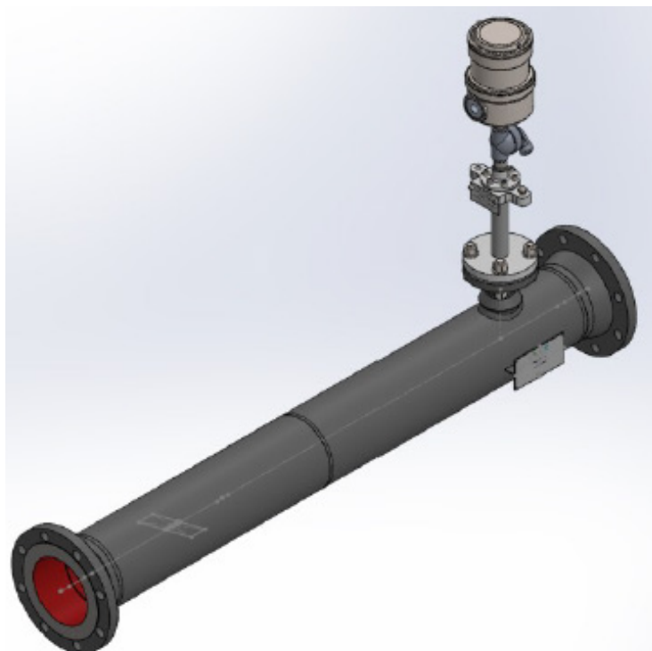
Figure 2-14: Installation into Smaller Pipe through a Pipe Bend
