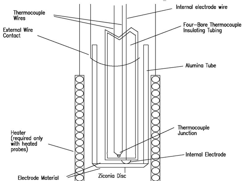
Figure 2-2: Zirconia Sensor Assembly
