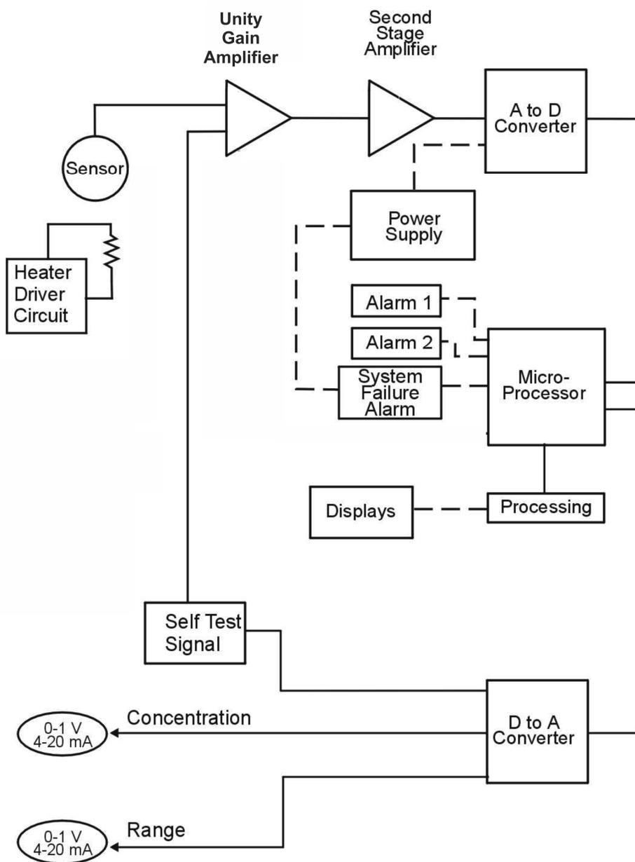
Figure 2-5: Electronic Block Diagram
