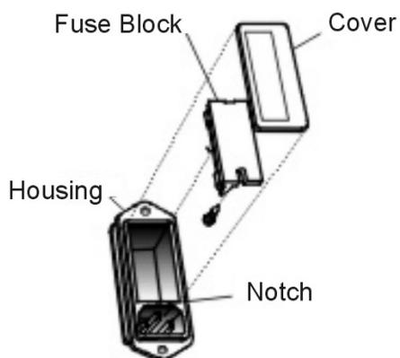
*Figure 5-1: Removing Fuse Block from Housing*
