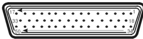
*Figure 3-4: Equipment Interface Connector Pin Arrangement*
