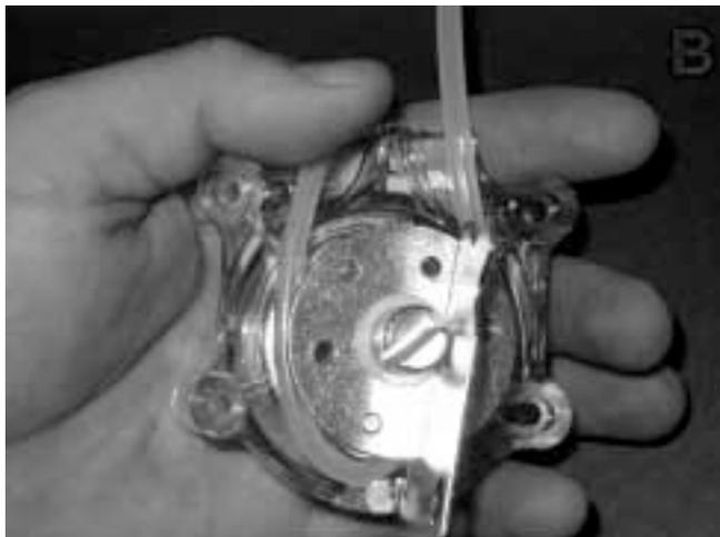
3. Place tubing in the right groove and against the first two rollers.
