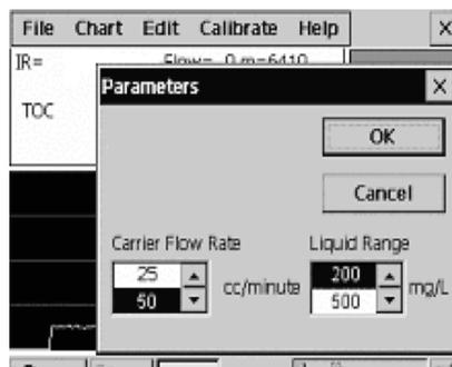
This is the Parameters menu from which the analyzer may be configured to suit the requirements of the operator
