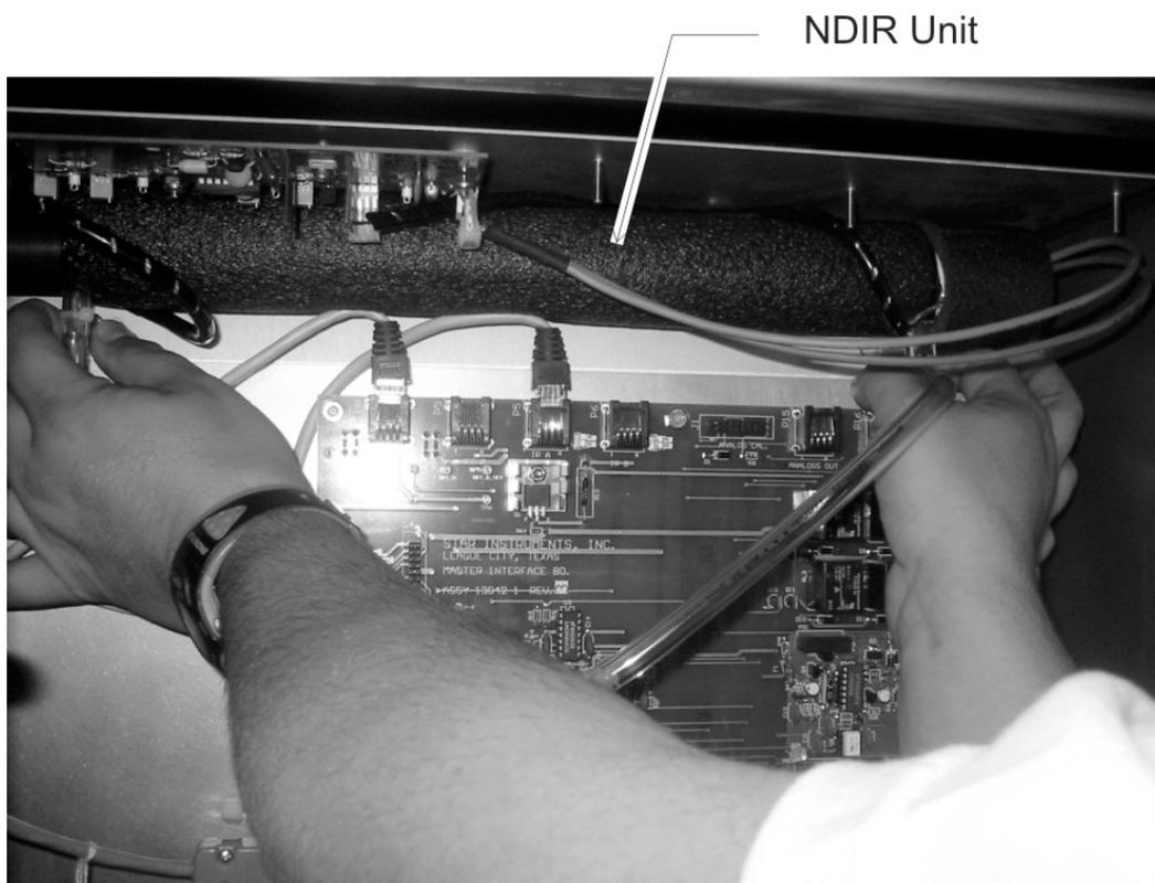
*Figure 5-4: Removing the NDIR Unit P/N ST36000*
