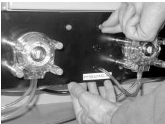
4. Remove two thumbscrews for pump panel removal.
