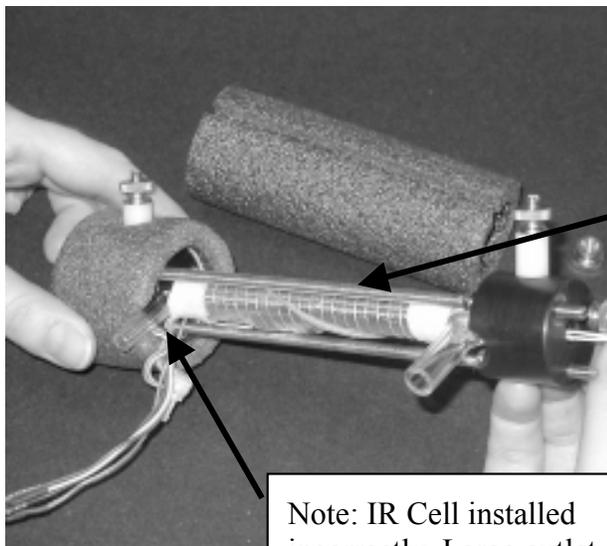
Note: IR Cell installed incorrectly. Large outlet port MUST go into Detector Assembly (left)
