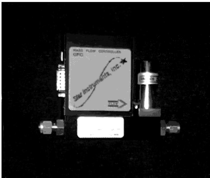
Figure 5-11: Mass Flow Controller
