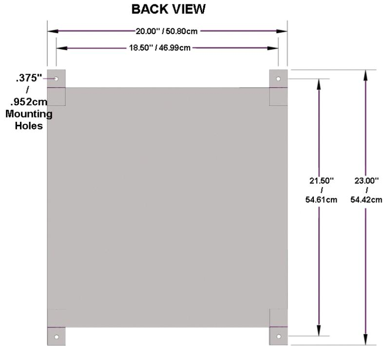
Figure 3-1: Analyzer Dimensions
