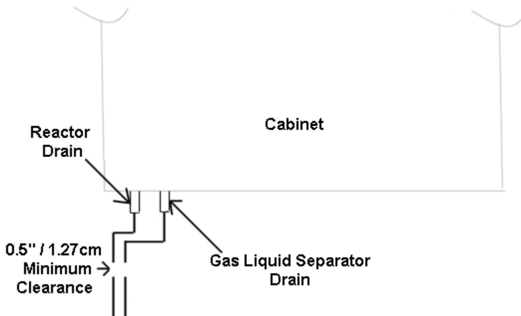
Figure 4-1: Drain Connections
