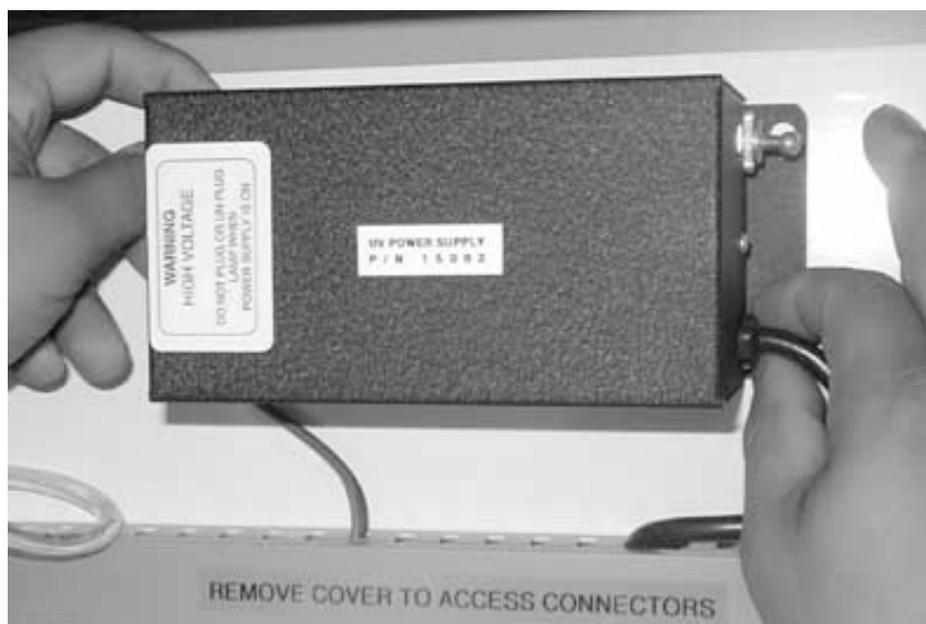
Figure 5-10: Removing the UV Power Supply
