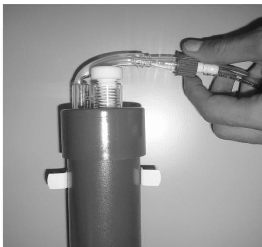
*Figure 5-1: Disconnecting Tubing from Reactor*
