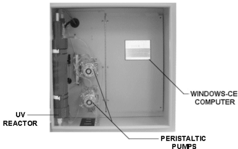
*Figure 1-1: The Model 6750 TOC Analyzer (Front door removed)*
