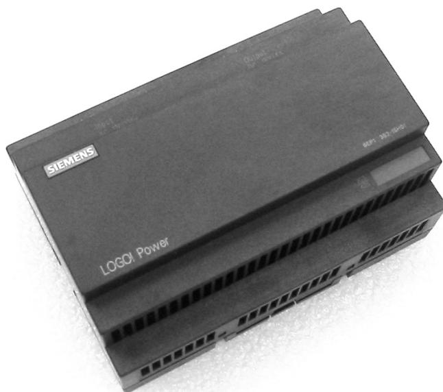
*Figure 5-6: DC Power Supply Module*
