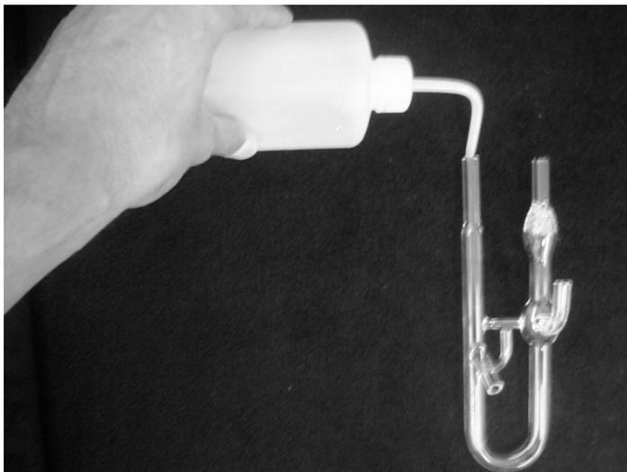
*Figure 4-2: Gas Liquid Separator D. I. Filling*
