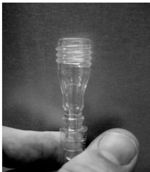
*Figure 5-2: IR Calibration Adapter P/N ST20026*
