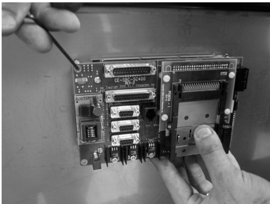
*Figure 5-7: Replacing CE Computer*
