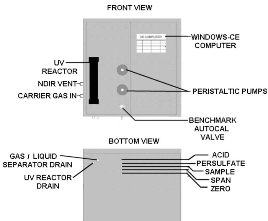
Figure 3-5: Gas and Liquid Connections to the Analyzer
