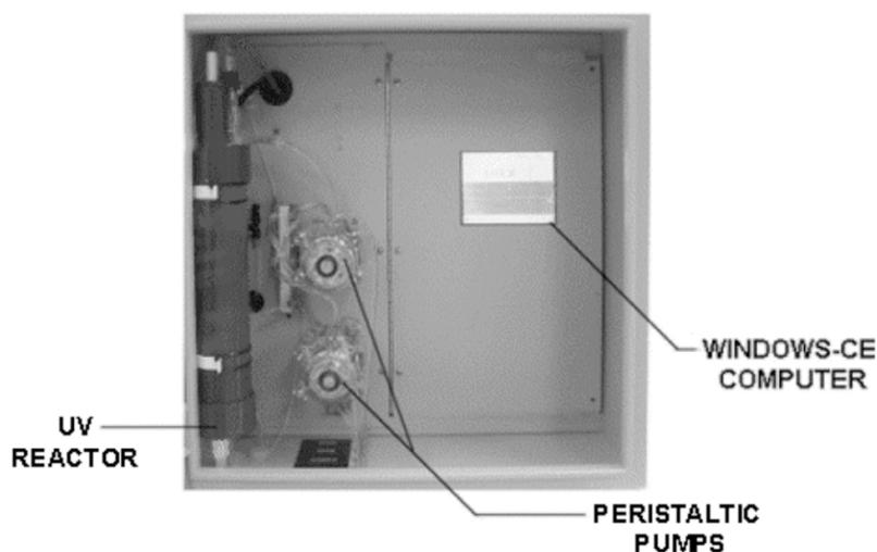
*Figure 3-3: Internal Components of the Model 6750 Analyzer*
