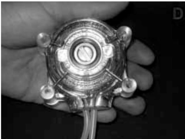
11. Position the other end bell on top and press the end bells together.
