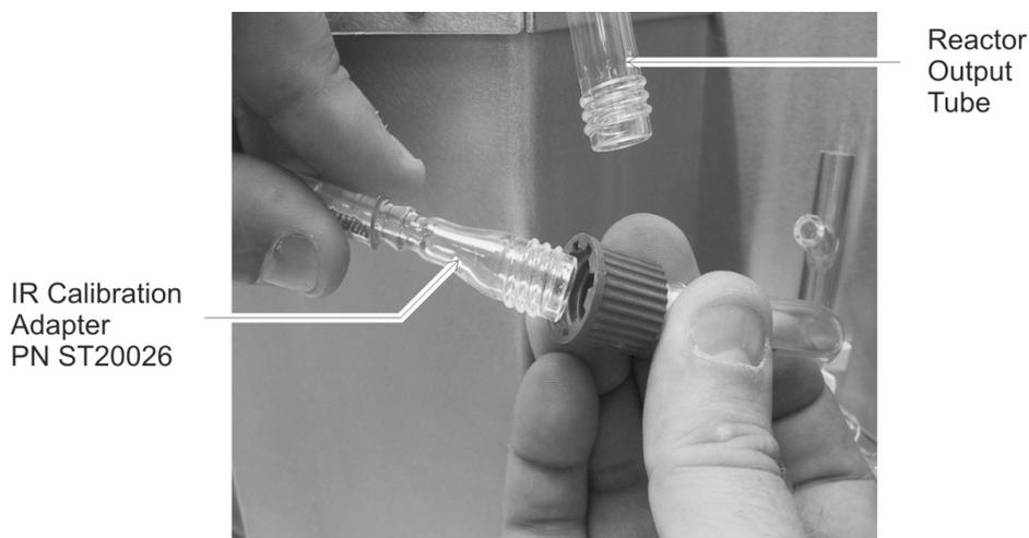
*Figure 5-3: Installing Calibration Adapter*
