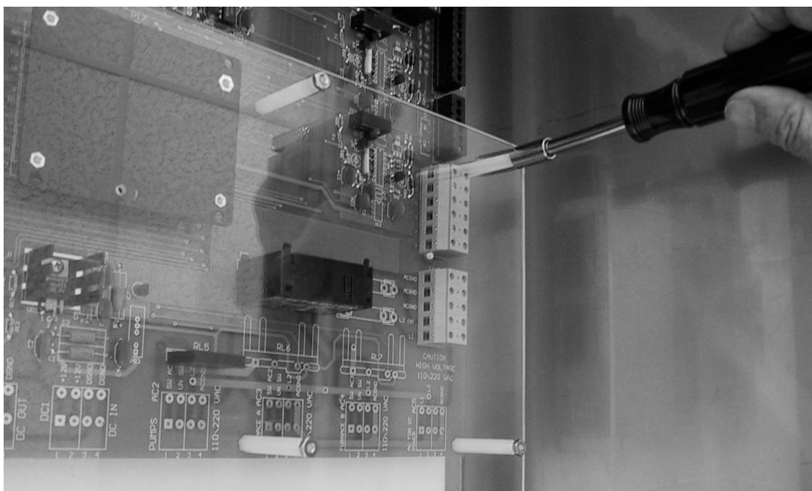
*Figure 5-5: Removing the Master Interface Board*
