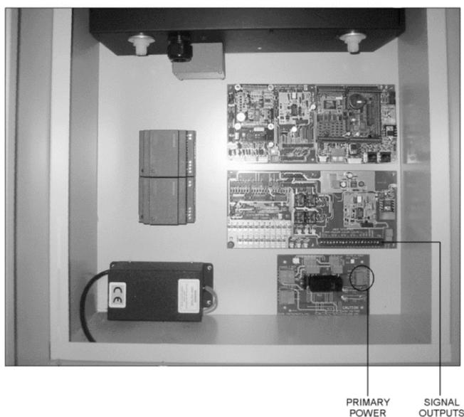
*Figure 3-4: Electrical Connections to the Model 6750*
