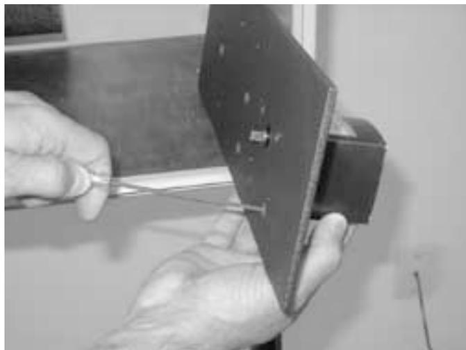
6. Remove 4 pump mounting screws for pump removal.
