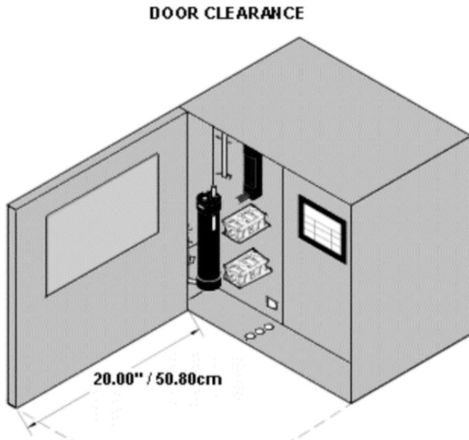
Figure 3-2: Required Door Clearance
