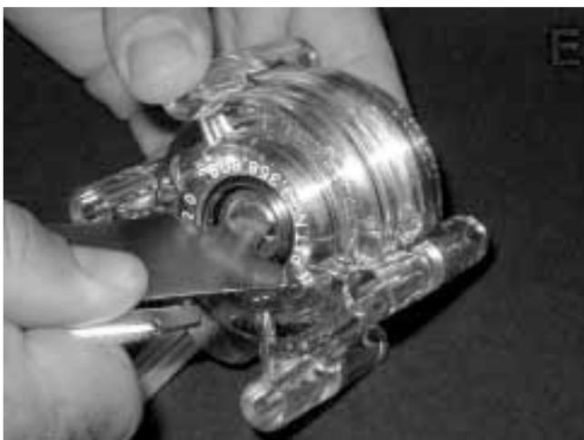
15. With key in slot on rotor shaft, turn key to align tang on rotor shaft with slot in motor drive shaft.
