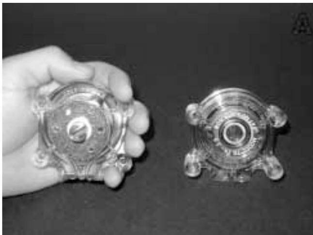
1. Separate the end bells (the pump head halves).
