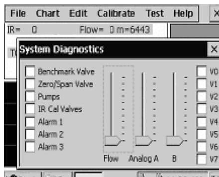
From this screen the operator may perform individual testing of components related to functionality and settings.
