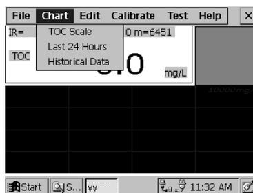
The display scale can be adjusted using the Select [TOC SCALE] item from the [CHART] menu. The following screen will appear.
