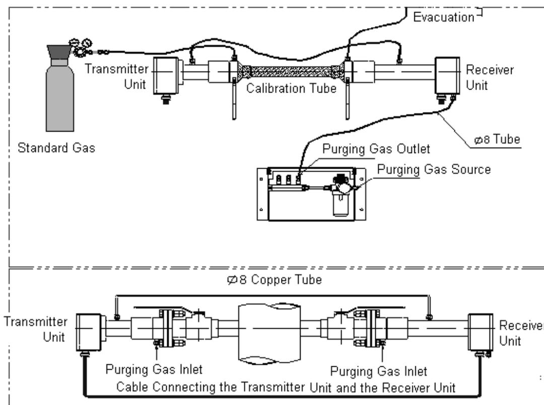
Figure 6.1 Schematic of the Calibration Setup
