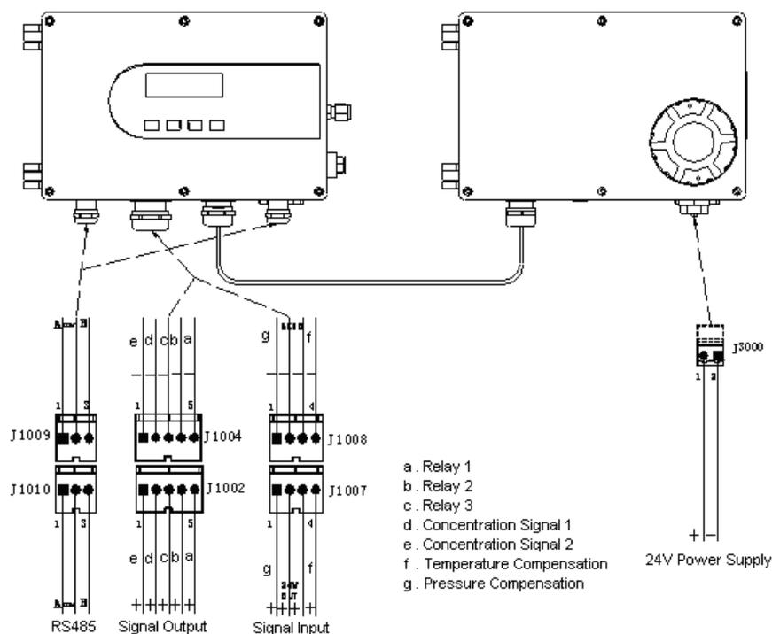
Figure 3.6: Electric Connection Diagram for the LGA-4000
