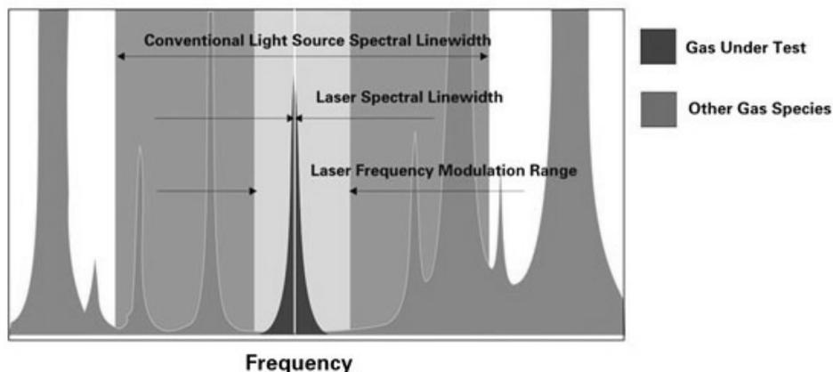
*Figure 2-5: Single Line Spectroscopy Principle*
