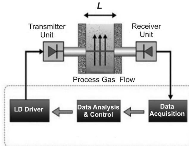
Figure 2-1: System Diagram for the LGA-4000 Series Analyzers
