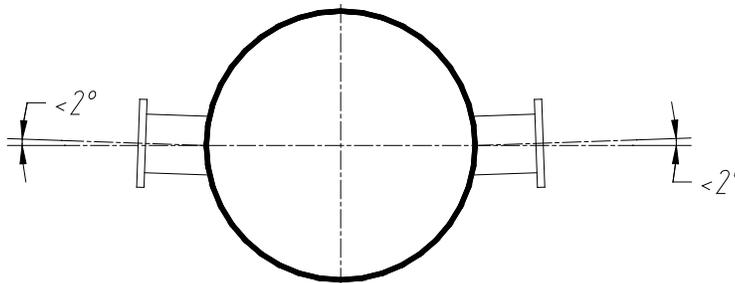
Figure 3.2: Allowed offset for welded flanges
