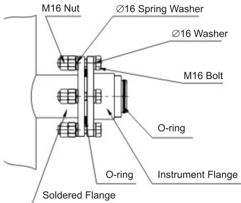
*Figure 3-3: Instrument Flange*
