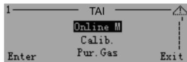
Figure 4-7: Alarm Indication on Main Setting Menu
