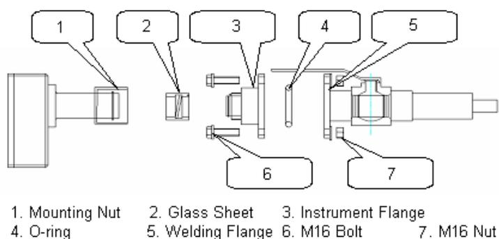
*Figure 3-7: Instrument Flanges and Hardware*
