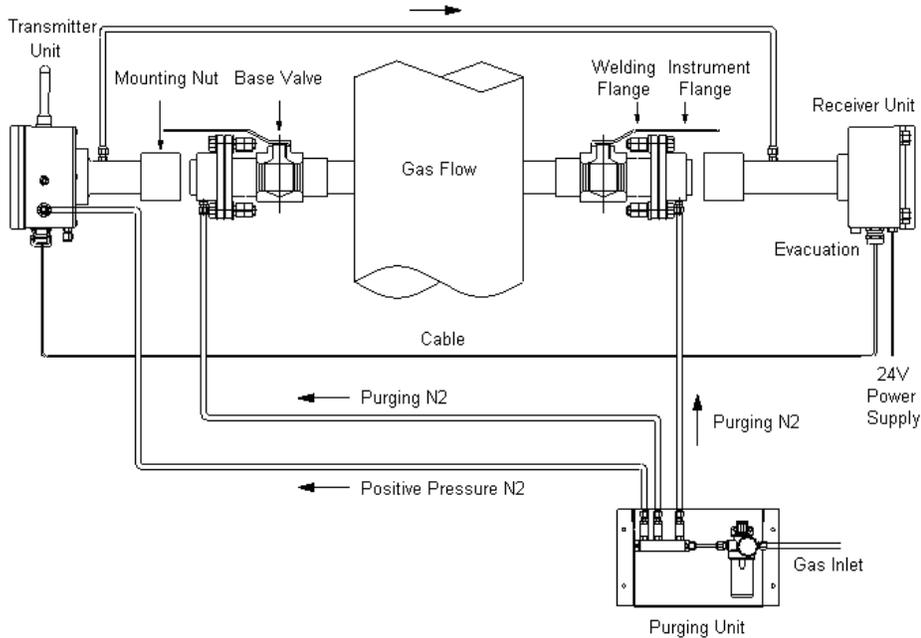
Figure 3-1: General Layout of the LGA-4000 Series Analyzer
